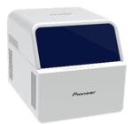
"Next-generation 3D-LiDAR Sensor" realizes highresolution long-distance measurement by utilizing SK Telecom's "1550nm wavelength laser transmitting module" and "Single Photon Detector".
