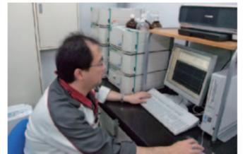
Measuring VOCs using a high-performance liquid chromatograph (HPLC) analyzer
