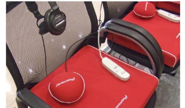
The body sensory audio system consists of a chair with a cushion and a pouch containing a vibrating unit. The system realistically conveys sound directly to the body as vibrations.
