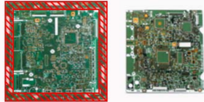
Waste circuit board (red shaded areas) were eliminated.
