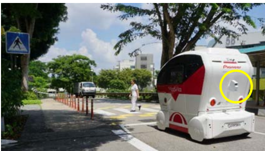
The autonomous shuttle bus equipped with four Pioneer's 3D-LiDAR sensors will realize a highly accurate object detection and self-localization
