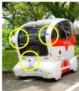
The autonomous shuttle bus equipped with four Pioneer's 3D-LiDAR sensors will realize a highly accurate object detection and self-localization
