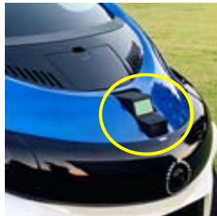
Renesas's demonstration car on which Pioneer's 3D-LiDAR sensor is mounted
