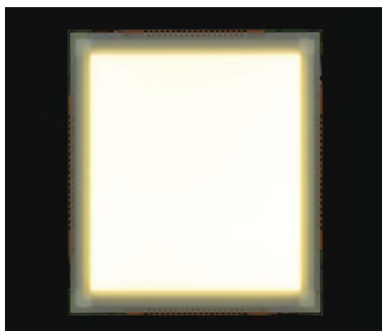
OLED lighting module with a wet coating process for a light-emitting layer
