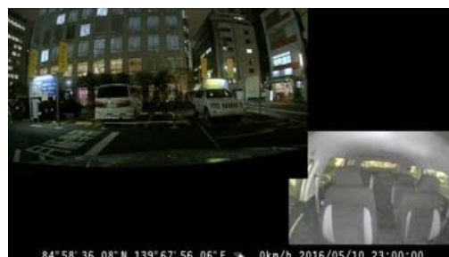
[Footage of both the inside and outside of the car is recorded when connected to the floor camera unit]
