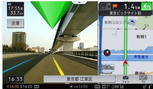
[Changing lane colors and sounding a warning tone to alert the driver]
