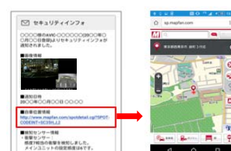
[Date and time, still image information, car position information and detection sensor information are notified]
