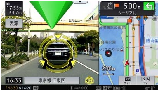
“Advanced Driving Assistance Functions” use image recognition technology
