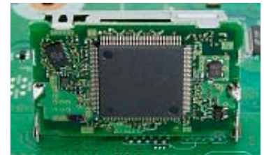
The "Regulus" system increases car positioning accuracy
