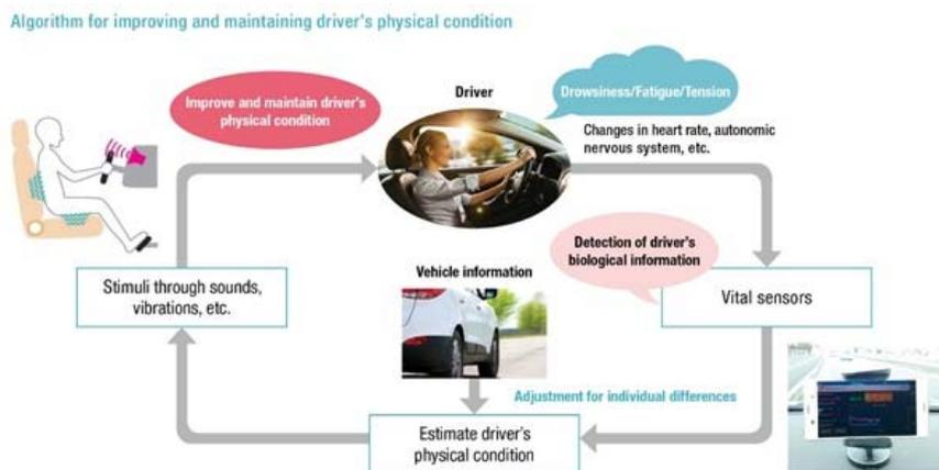
[Early detecting the drowsiness of a driver from the heart rate and improving and maintaining the level of alertness using vibration (conceptual image)]
