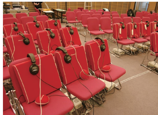
A cushion and pouch containing a vibrating unit that conveys sound directly to the body are installed at the concert halls.
