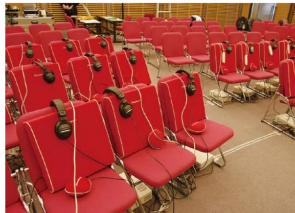
A cushion and pouch containing a vibrating unit that conveys sound directly to the body are installed on the seats at the concert halls.
