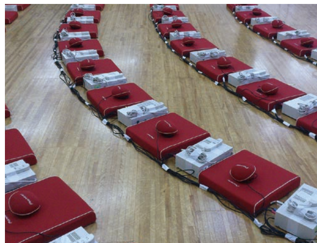
A cushion and pouch containing a vibrating unit convey sound directly to the body. (School for the Deaf in Tokyo)
