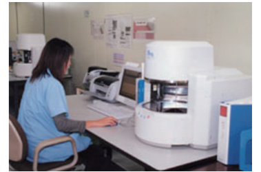
Using a fluorescent X-ray analyzer to rigorously check for hazardous substances
