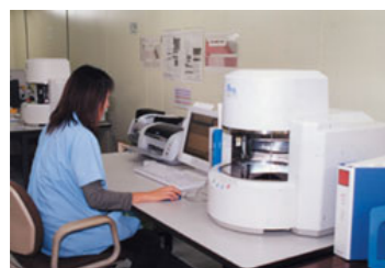
Using a fluorescent X-ray analyzer to rigorously check for hazardous substances
